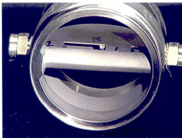
P/N 3202222-1 bleed air check valve.
