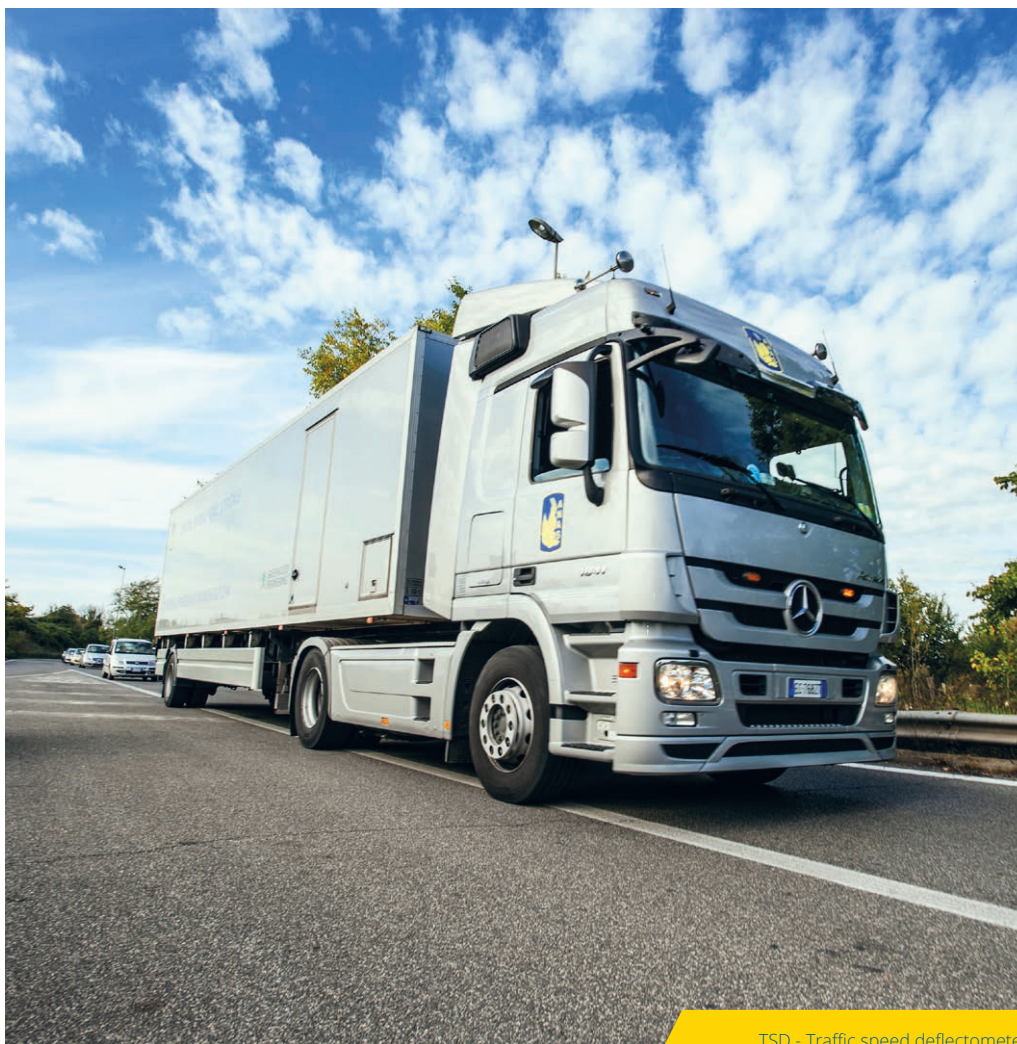
TSD - Traffic speed deflectometer
